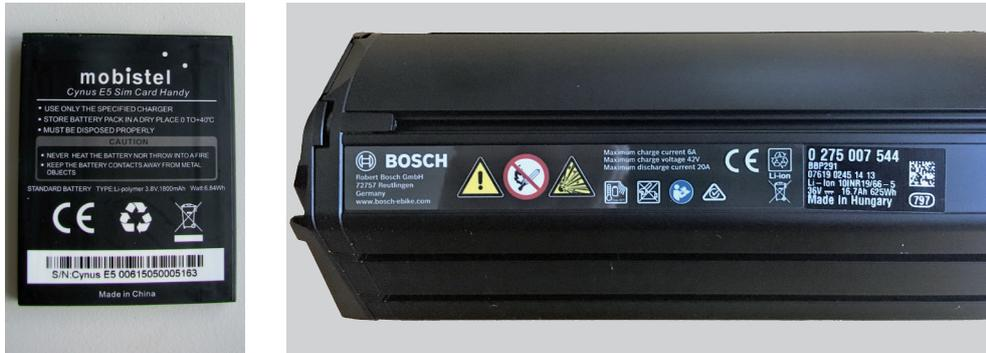
Abb. 21: Lithium-Akkumulatoren (links Smartphone, rechts E-Bike)
